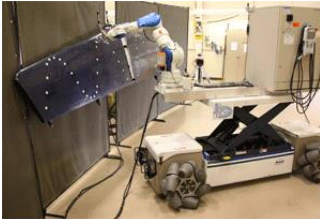
Mobile robot working on aircraft wing, courtesy Southwest Research Institute.
