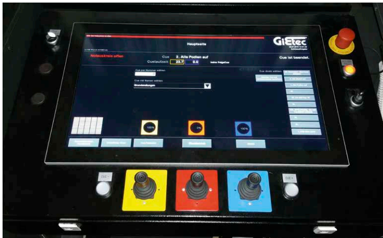
Two identical, multi-purpose Stage Controllers from Gietec, based on a Panel PC 900 with a projected capacitive 24" touch screen serve as control consoles for the 55 movable platforms that transform the stage during every performance of The Wyld .
