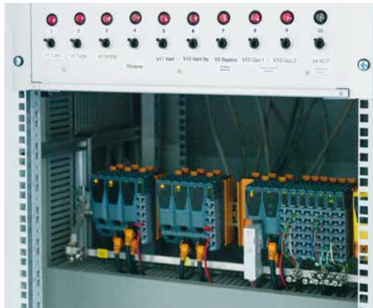
To determine whether the satellites are prepared for deployment in space, they are tested in a manual thermal vacuum chamber. This chamber is operated using a controller and other modules from B&R's X20 system.
