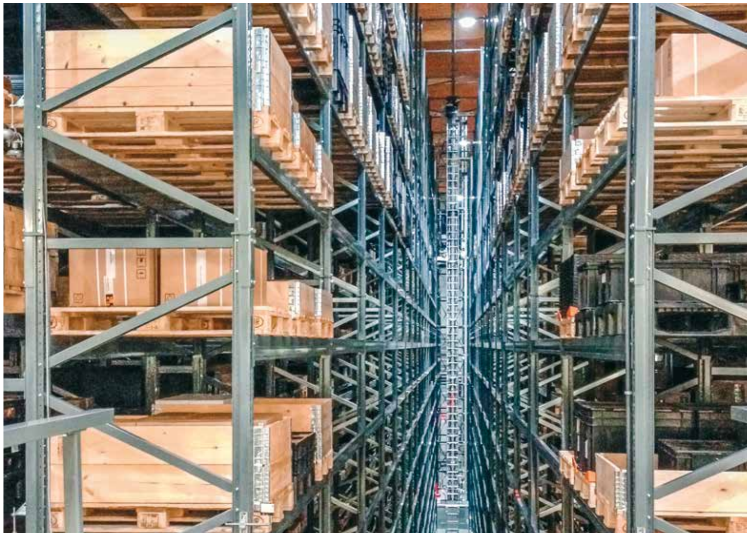
BSR's production halls are fully networked. The ERP system has direct control of the storage and retrieval vehicles in the high bay warehouse and automatically optimizes production logistics.
