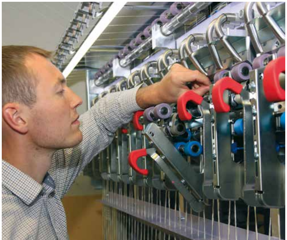
Michael Lau checks the quality of the roving in the open drafting system.
