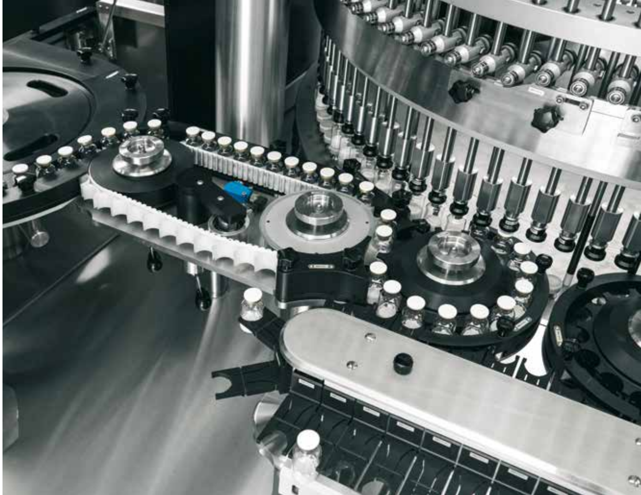
High precision at high speeds: An InnoScan inspection machine typically inspects 10 to 25 different attributes on filled vials – at speeds approaching 650 vials per minute.
